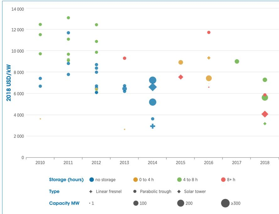
Figure 16: Total installed costs of CSP plants by technology and storage capacity [107].
